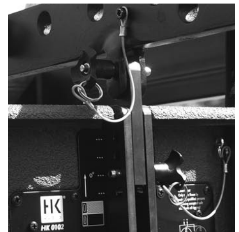
Figure 10: Connector component attached to the top rigging frame for a 0° curving angle
