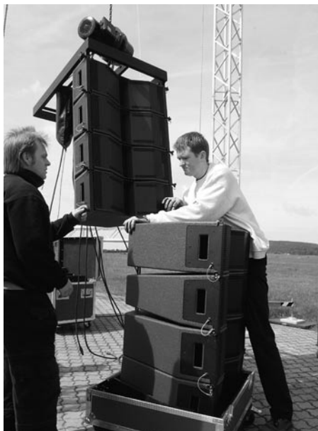
Figure 16: Hoisting the top four COHEDRA® mid/high enclosures
