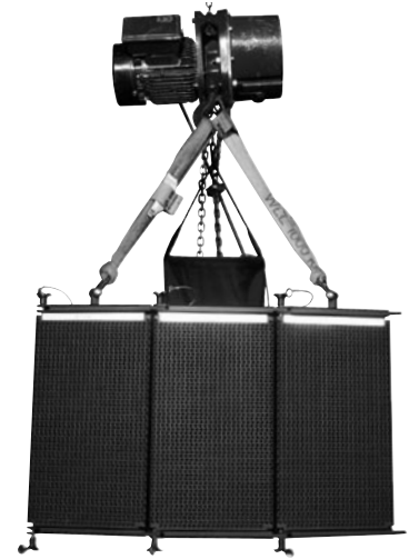
Figure 10: Horizontal array comprising three CDR 108 Cs
