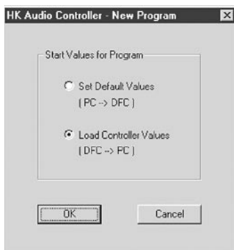
Figure 5: Loading and setting controller values
