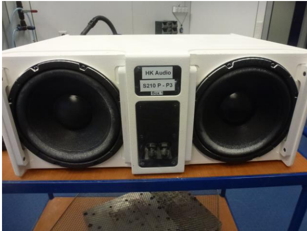
3. UUT 1 after IP 6X, back side, protective grill removed
