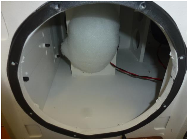
5. Back speaker expanded; no ingress of dust visible
