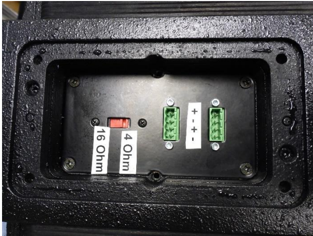
15. Connection Board no ingress of water
