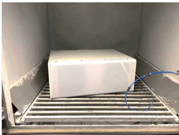
1. UUT 1 in the dust chamber before IP 6X
