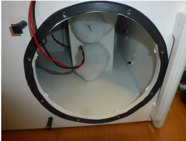
7. Front speaker expanded; no ingress of dust visible
