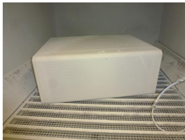
2. UUT 1 in the dust chamber after IP 6X
