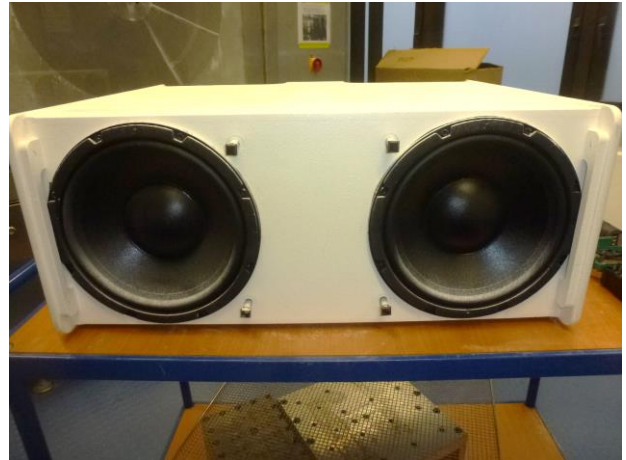
4. UUT 1 after IP 6X, front side, protective grill removed
