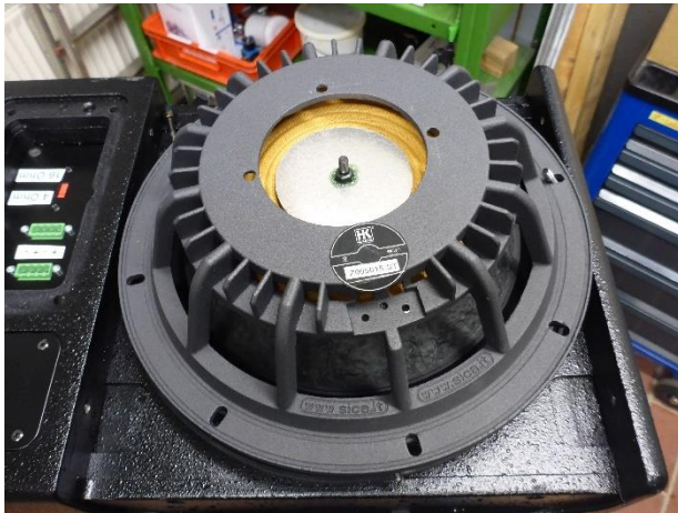
17. Speaker expanded; no ingress of water visible
