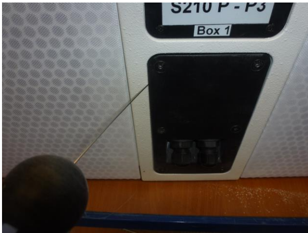
11. UUT 1, no ingress with the Ø 1 mm test probe possible
