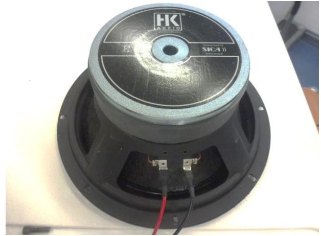
8. Front speaker expanded; no ingress of dust visible
