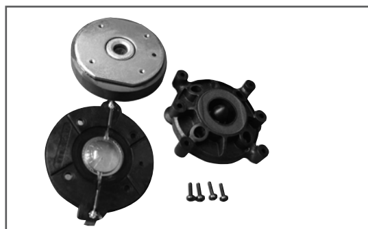
Fig. 38: Voice coil removed from the CAD 208 HF driver
