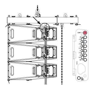
**6** Remove the quick-release pins of the lowest M/H unit on the C-WB and lift the array until the entire load is suspended from the lifting accessories and link pins.
