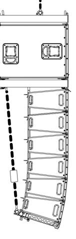
**7** You may fasten ropes to the pull-back frame's attachment points to tie the array to truss bars or the like to prevent it from twisting in the wind.
