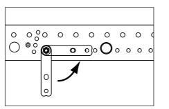
Note: Make sure the flap is in the parked position and fixed in place with the pin.
