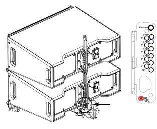
**14** Hook the red tensioning end of the tensioning strap into the CRF-PB's rear shackle and connect the loose and tensioning ends of the strap.
