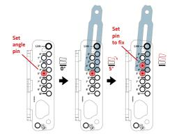
Fig: A 5° angle in fixed mode (ground stack)
