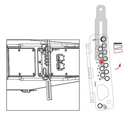
**9** Insert the fix pin to secure the connection between these two M/H units.
