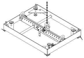
**3** Lift the rigging frame until there is sufficient clearance for the first C-WB wheel board to slide under it.
