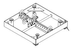
The multifunctional CRF-60 serves as a rigging frame for C 6, C 8 and C 10  $\,$  M/H units, or for ground stacks.
