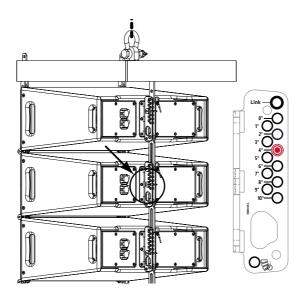
Heads up: Remove and replace angle pins only when the array is suspended and there is no load on them; otherwise, you run the risk of pinch/crush injuries. 8 Raise the array just high enough for the next C-WB to slide in below it.
