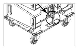
7 Now set all mid/high units' angle pins to the desired position on the angle plate (see the pictured example for a 4° angle).
