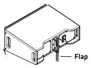
The flap links the individual components and is always attached to the angle plate of the bottom M/H unit in compressed or fixed mode. The M/H units C 6 and C 8 may be tilted by up to  $10^{\circ}$  in  $1^{\circ}$  steps. The maximum angle for the C 10 is  $6^{\circ}$ .
