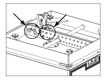
The C-GSA has two rows of holes offering the following angles: –6° to –16° or –18° to –20°.
