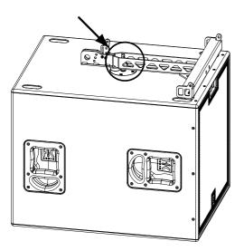
**3** Attach the COSMO M/H unit to the CRF-PB pull-back frame.
