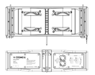
Driven via a passive x-over, this two-way M/H line array unit is loaded with two 6.5" midrange woofers and a 1.4" HF driver fronted by a Multicell Transformer (MCT). With 100° horizontal directivity, it is perfect for short throw distances.
