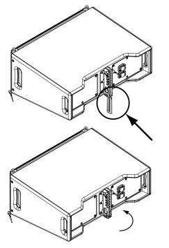
**12** Insert the two quick-release pins to attach the CRF-PB to the lowest M/H unit in the array.
