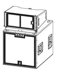
**4** You can set the M/H unit's angle on the CRF-PB to  $-5^{\circ}$ ,  $-3^{\circ}$ ,  $0^{\circ}$ ,  $+2^{\circ}$  or  $+5^{\circ}$ .
