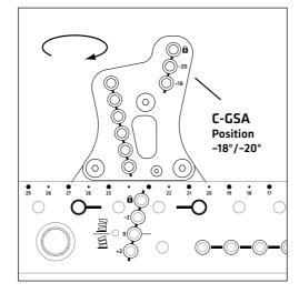
**2** Attach the M/H unit to the rigging frame's attachment points.
