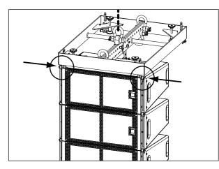
**5** Attach the rigging frame's flap using the hole labeled link in this M/H unit's rear angle plate. Now insert the loose end of the tensioning strap with the crane hook into the rigging frame's lower shackle.
