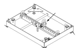
2 Connect the chain hoist or other hoisting equipment to the C-PPA's shackle and lift the rigging frame to a convenient working height.
