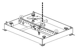
Note: The shackle for securing the tensioning strap is only required for the adapter frame (see step **6** above).
