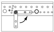
Heads up: Flip the flap back for ground stacks with the CRF-60 or CRF-80.
