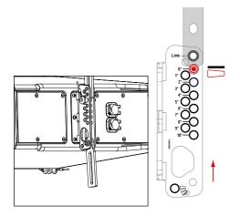
Note: The angle between the frame and the first M/H unit should be 0°, the same angle as used in GLL data sets.
