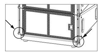
13 Insert quick-release pins to attach the pull-back frame's spacer adapter at the proper position in the M/H unit's angle plate.
