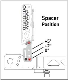
Setting the tilt angle with the M/H unit's flap:
