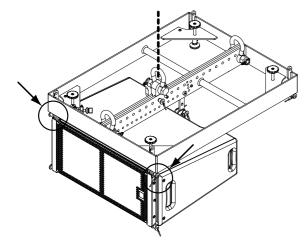
**5** Insert the rigging frame's flap into the M/H unit's angle plate and lift it until the flap meets the angle pin.
