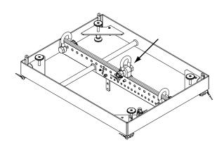
**2** Connect the chain hoist or other hoisting equipment to the C-PPA's shackle.
