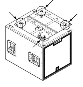
4 Attach the M/H unit to the rigging frame's attachment points.
