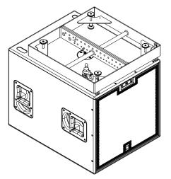
**3** Level the rigging frame with the four adjustable feet. The spirit level built into the CRF-60 or CRF-80 serves this purpose.
