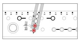
**6** Connect all other M/H units required for the ground stack in fixed mode.
