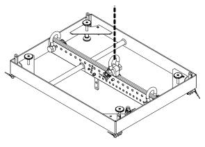
**3** Insert the individual angle pins at the desired position and remove the fix pin from the M/H unit's angle plate before attaching each M/H unit.
