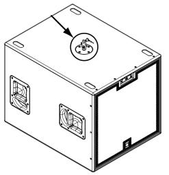
2 Place the CRF-80 or CRF-60 on the subwoofer and insert the quick-release pin to attach it to the C-M20 adapter.
