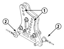
Holes to adjust the tilt angle
