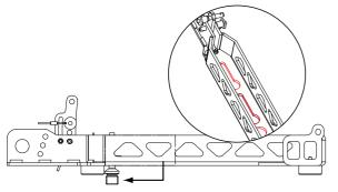
2 Set the CRF-PB on the CS 118 or CS 218; then screw the C-M20 adapter into the subwoofer's M20 threaded insert. The pretensioning, due to screwing the adapter into the sub's threaded sleeve, affixes the CRF-PB to the top of the subwoofer.
