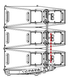
**15** Engage the tensioning strap's ratchet until all flaps are fully attached to the angle pins and you arrive at the desired preset curvature.
