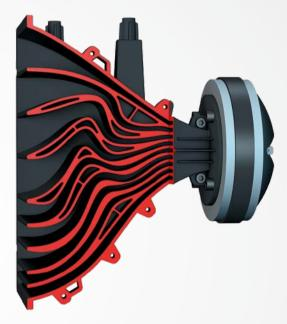
Here's a simplified run-down of how it works: the MCT splits the wavefront into nine small wavefronts. Each of these partial waves is directed through the flaring duct of a horn of different length and mouth size. These horns don't have acres of real estate that can cause interference, so the only distortion they generate is beyond the range of human hearing. This increases useful sound pressure by up to 10 dB.
