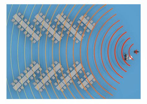
POLAR 8 boasts wide dispersion and homogeneous volume distribution and is less prone to feedback, making it easy to position.
