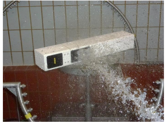
18. UUT during IP X6
