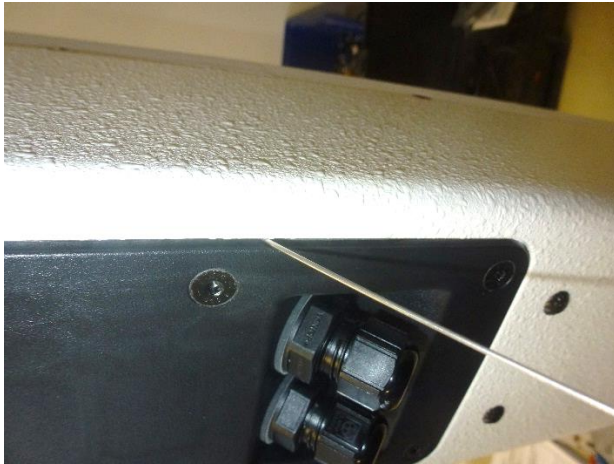
5. Penetration with the access probe \varnothing 1mm not possible
