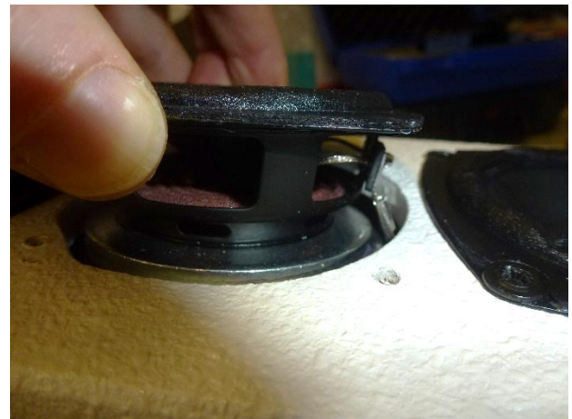
28. Speaker - no penetration of water visible
