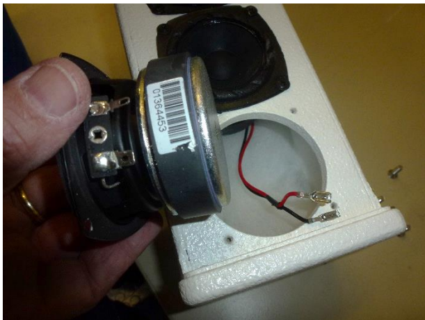
27. Speaker - no penetration of water visible
