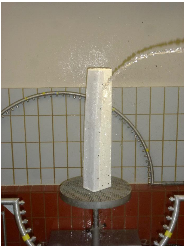
15. UUT during IP X5
