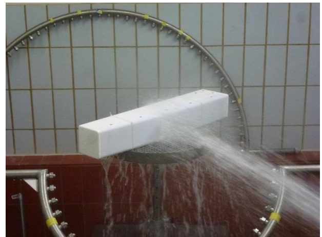
20. UUT during IP X6
