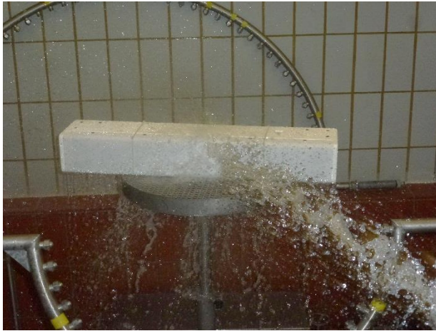
17. UUT during IP X6
