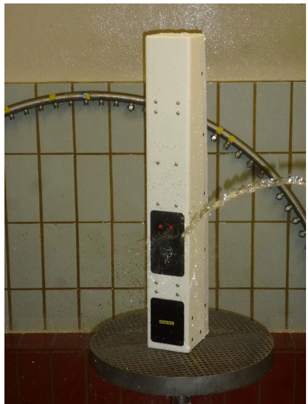
16. UUT during IP X5
