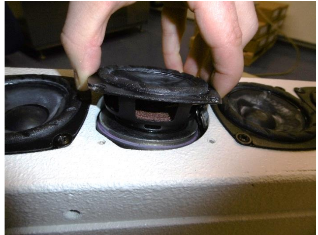
14. Speaker - no penetration of dust visible
