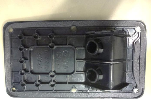
22. Cover connection box – no penetration of water visible
