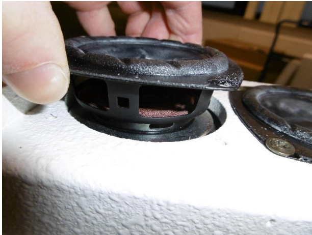
13. Speaker - no penetration of dust visible
