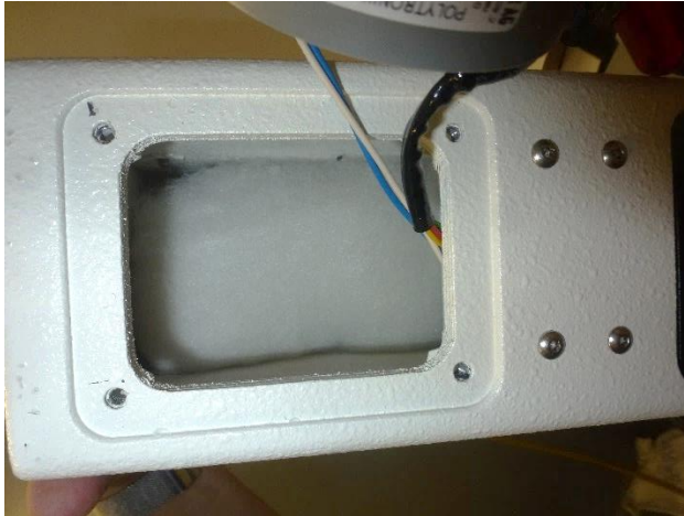
21. Transformer box – no penetration of water visible
