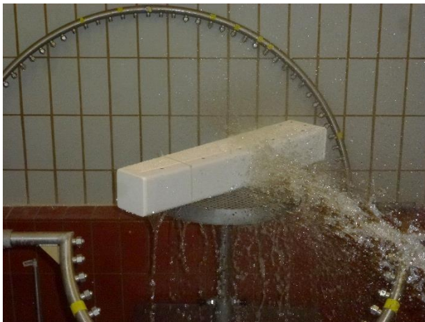
19. UUT during IP X6
