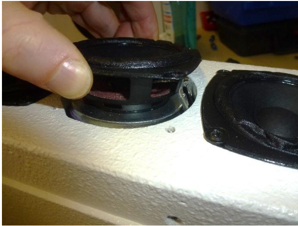
25. Speaker - no penetration of water visible
