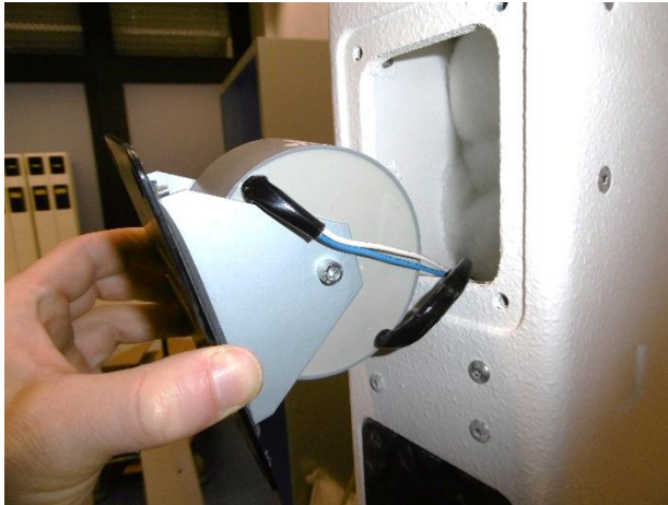
9. Transformer box – no penetration of dust visible
