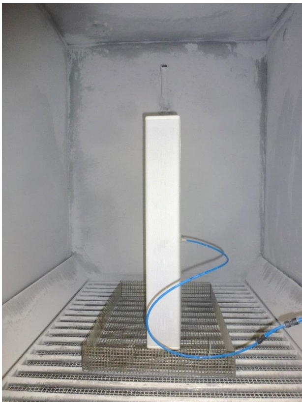
7. UUT before IP5X / 6X in the dust chamber
