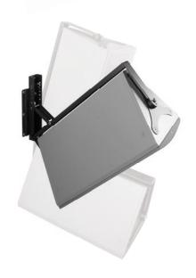
The VR2-10810 is a professional-grade, full-range speaker system housed in a bass reflex enclosure with a passive crossover, 8" bass/midrange woofer and a 1" high-frequency driver coupled to a CD horn.
