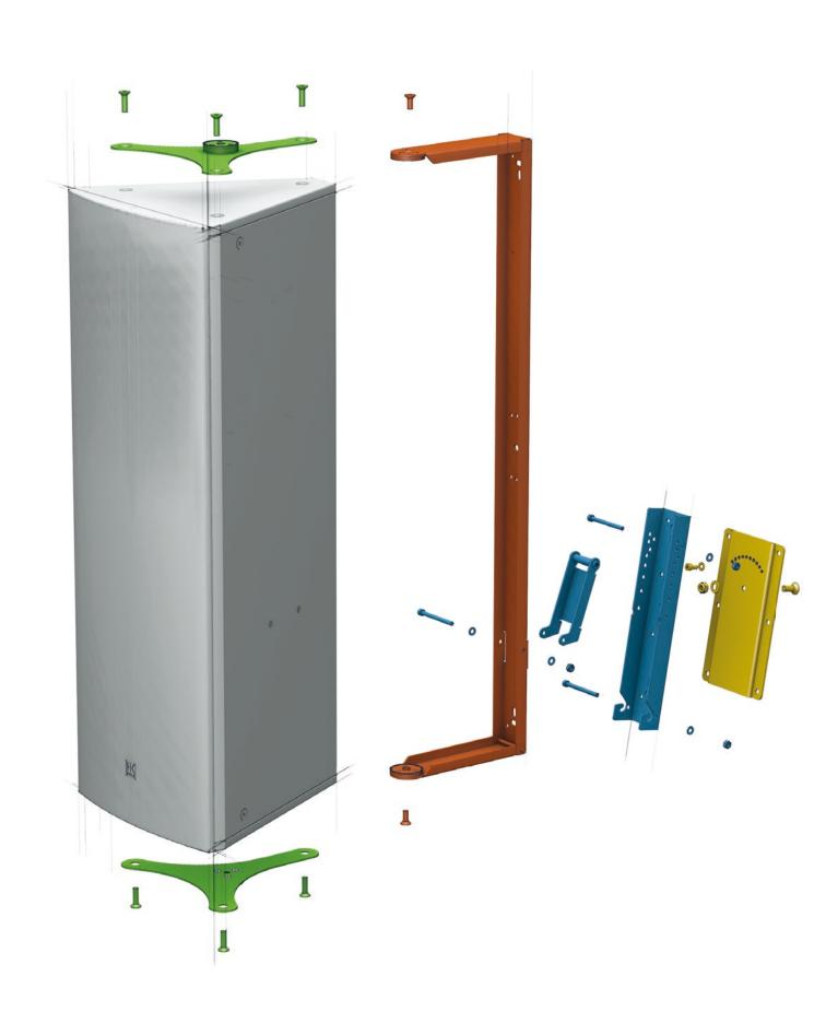
The U-bracket comes with a wall-mount plate and a tilt unit serving to install the speaker at any desired angle.
